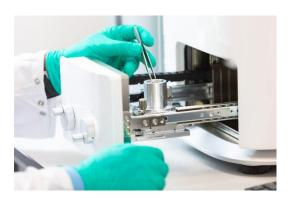
The centre has therefore purchased the latest in benchtop SEM technology from Nikon. The JCM-6000Plus "NeoScope<sup>TM</sup>" is a
