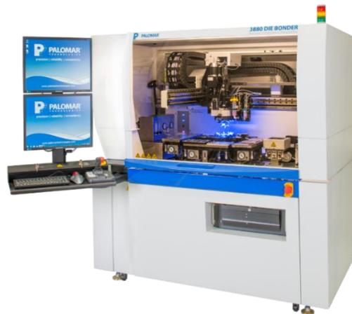
The **3880** offers capabilities that would ordinarily require at least four separate machines (eutectic die bonding, material dispensing, flip chip and UV bonding).
